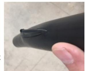
Vincent also has shallow-buried several HDPE welded pipe systems in recent years. Shallow bury systems are usually with 2 feet of the soil surface (not below the frost line). Shallow bury appears to normalize pipe temperatures and thus appears to avoid the entrained air rupture issues associated with some above ground systems. However, shallow bury systems can still get a vacuum lock associated with high spots on occasion and air gaps are still recommended.
